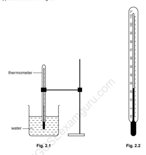
(a) Record the value of room temperature  $\theta_{\rm R}$  shown on the thermometer in Fig. 2.2.
